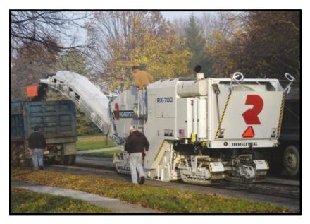
The RX-700 is a 700 horsepower cold planer available with either three or four track assemblies. This versatile machine allows contractors to cut up to 14" (35.6 cm) deep with widths of 6'7" (2 m), 7'2" (2.184 m). The RX-700 offers contractors more versatility and productivity. A 36" inch front load-out conveyor, with 60° swing to either side, provides ample loading capacity.
