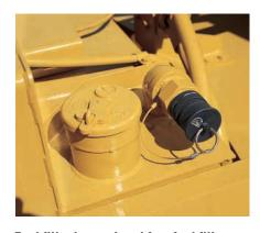
Fuel fill tube, optional fast fuel fill attachment, and fuel tank are positioned away from debris and easily reached.
