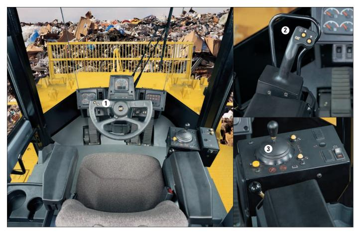
The 836G benefits significantly from the dramatic reduction in operator motion effort provided by Assist steering, STIC steering, and hydraulic blade controls. These features make the 836G the easiest operating machine in its size class.
