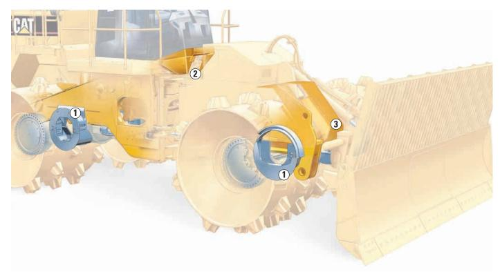
**The Cat Axle Guard System** protects final drives, planetaries and seals from damage caused by wire, cable, plastics or other materials which can wrap or become packed around axle components.
