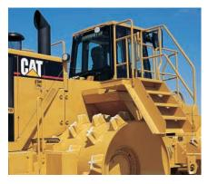
**Rear access walkover stairway** provides easy access to operator's station. Optional swingout stairway, provides for unparalleled access for clean-out, service and maintenance.
