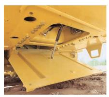
Electrically actuated engine and power train guards help prevent trash build-up and shield components from demolition debris, trash, wire, rebar and harmful chemicals.
