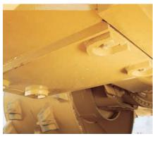
**Bolt protection** is provided on machine bottom to prevent premature wear out.
