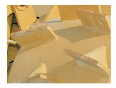
**Self-cleaning Chopper Wheels** (optional) are designed to deliver maximum compaction and traction in landfill work.
