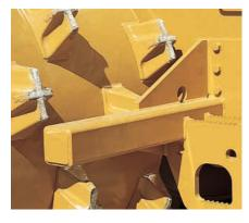
**Striker bars** are in front and behind the rear wheels, and behind the front wheels. They provide substantially improved protection from trash that can be thrown or carried by the wheels. The front also provides for access to the fuel tank in front frame.
