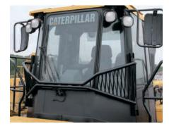
**Optional Front Window Guard.** An all new, tubular steel guard across the bottom of the front cab glass prevents large debris from damaging the lower portion of the front windows.
