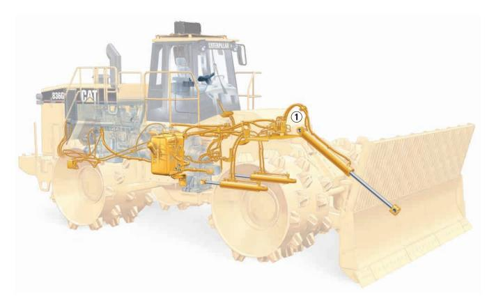
**Revolutionary electro-hydraulic control system** provides low-effort fingertip control. Floor-mounted control pod lever sends electrical signals to a pilot valve mounted on the front frame. This moves the sound, heat and effort caused by a hydraulic valve out of the operator's station.
