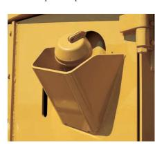
**Hydraulic tank** is guarded to resist damage. Oil sight gauge is visible for easy checking.
