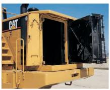
Hydraulically driven demand fan automatically adjusts fan speed for optimum cooling, resulting in reduced power draw on the engine, better fuel efficiency, and more power for the hydraulics and rimpull.
