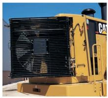
The Reversing Demand Fan is a speed controlled, hydraulic fan that provides maximum cooling efficiency. Power is directed through the fan system only when it is needed and reverses automatically to purge debris. (Pressing rocker switch in cab may also manually reverse fan.)
