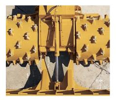
**Front frame guards** prevent trash buildup inside the frame that could damage hydraulic lines. The lift lines are in a higher location where damage from debris is less likely.
