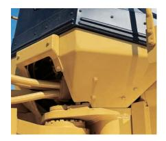
**Cab bottom guard** protects hoses and wires beneath the cab from damage due to flying debris and waste.
