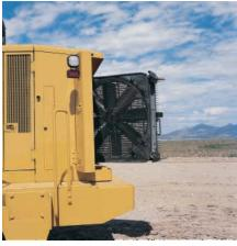
Auto-Reversing, Hydraulically-Driven Demand Fan. The demand fan automatically adjusts fan speed for optimum cooling, resulting in reduced power draw on the engine, better fuel efficiency and more power for the hydraulics and rimpull.
