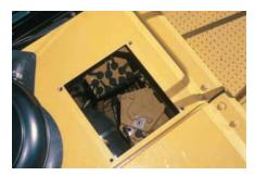
**Service Access.** Scheduled maintenance points are well within reach and the transmission (ECPC) remote pressure taps are now located behind the cab, under the platform door for easy access.
