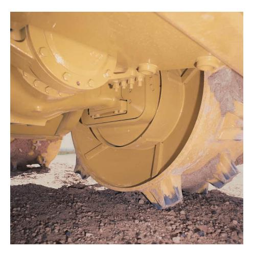
**Cat Axle Guard System.** The Cat Axle Guard System protects the final drives, planetaries and seals from damage caused by wire, cable, plastics or other materials which can wrap or become packed around axle components.
