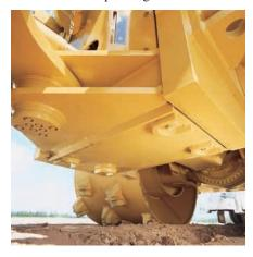
**Bolt Protection.** Located on the machine bottom, bolt protection prevents premature wear.
