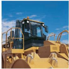
**Optional Front Window Guard.** An all new, tubular steel guard across the bottom of the front cab glass prevents large debris from damaging the lower portion of the front windows.
