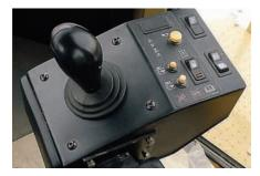
**Automatic Blade Positioning (ABP).** The patented ABP system is intended to lower fatigue, increase comfort and make the operator more productive.
