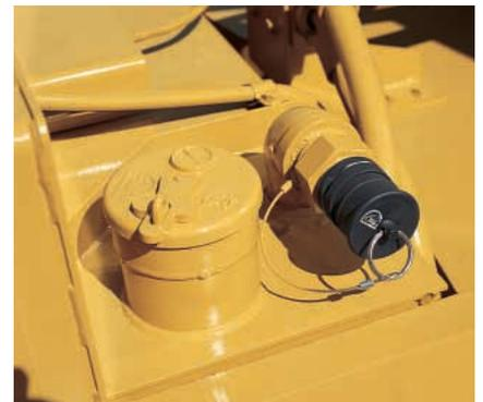
**Fuel fill tube, optional fast fuel fill attachment, and fuel tank** are positioned away from debris and easily reached.
