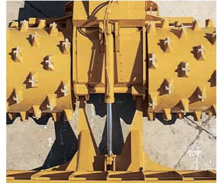
**Front frame guards** prevent trash build-up inside the frame that could damage hydraulic lines. The lift lines are in a higher location where damage from debris is less likely.
