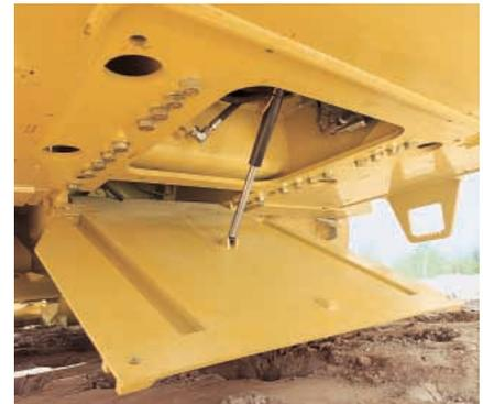
**Electrically actuated engine and power train guards** help prevent trash build-up and shield components from demolition debris, trash, wire, rebar and harmful chemicals.
