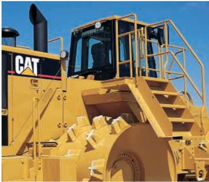
**Rear access walkover stairway** provides easy access to operator's station. Optional swingout stairway, provides for unparalleled access for clean-out, service and maintenance.
