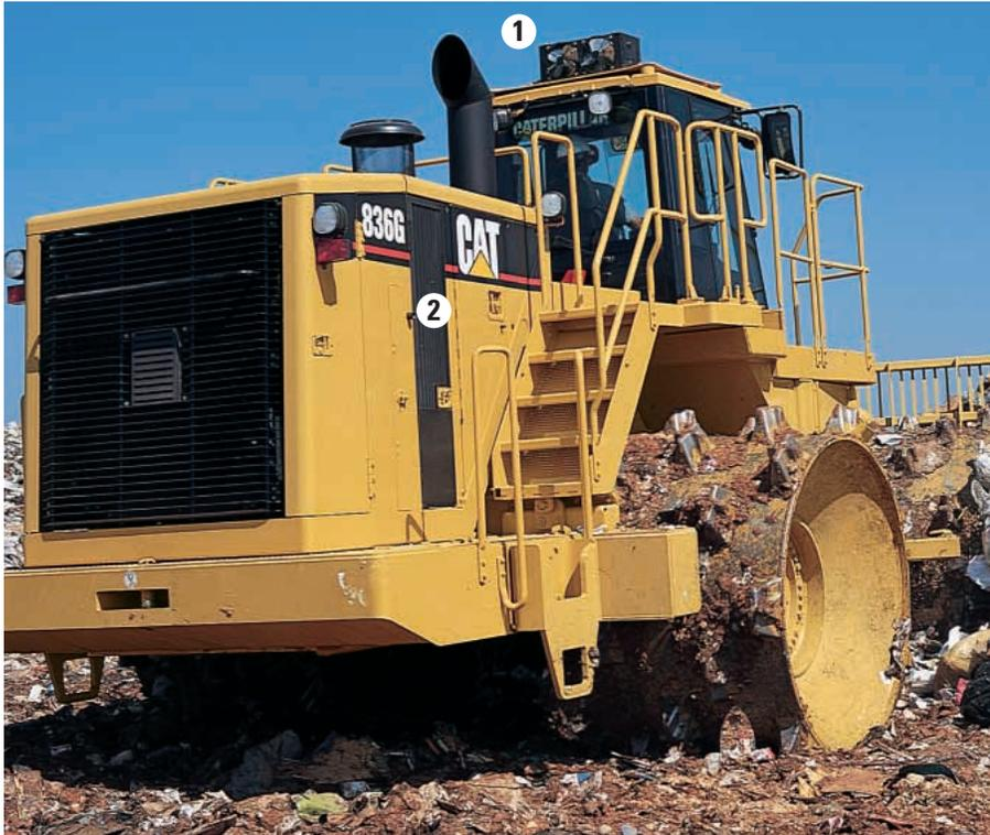
**The new separated fan and cooling system** on the 836G incorporates many trash resistant features, including an automatic reversing hydraulic demand fan, which reduces the chance of trash and debris entering the engine compartment. The system also reduces operating costs (fender cleanouts) and increases cooling capacity.
