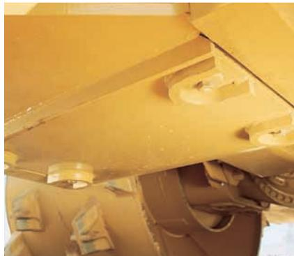
**Bolt protection** is provided on machine bottom to prevent premature wear out.
