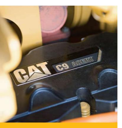
The D7E electric drive train is powered by a 235 hp Cat C9.3 engine with ACERT<sup>TM</sup> Technology. The engine utilizes a proven common rail fuel system for improved efficiency and fuel economy. Featuring the latest in Cat emissions reduction technologies, this engine meets U.S. EPA Tier III, EU Stage IIIa and Japan MLIT Step 3 emissions regulations.
