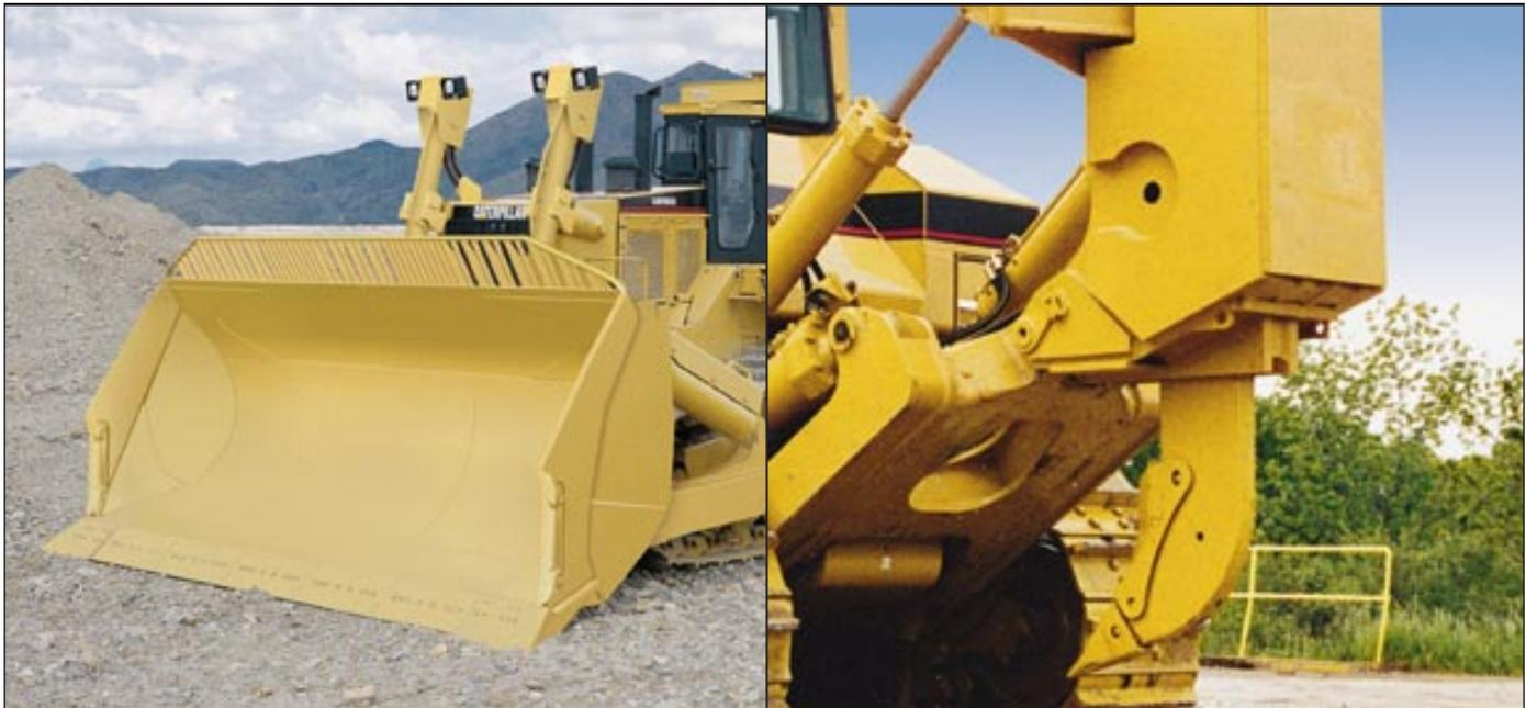
**Carrydozer Blade** carries material inside the blade curvature for maximum productivity. This increases the effective weight of the tractor which enables pushing a larger pile of material in front of the blade.
