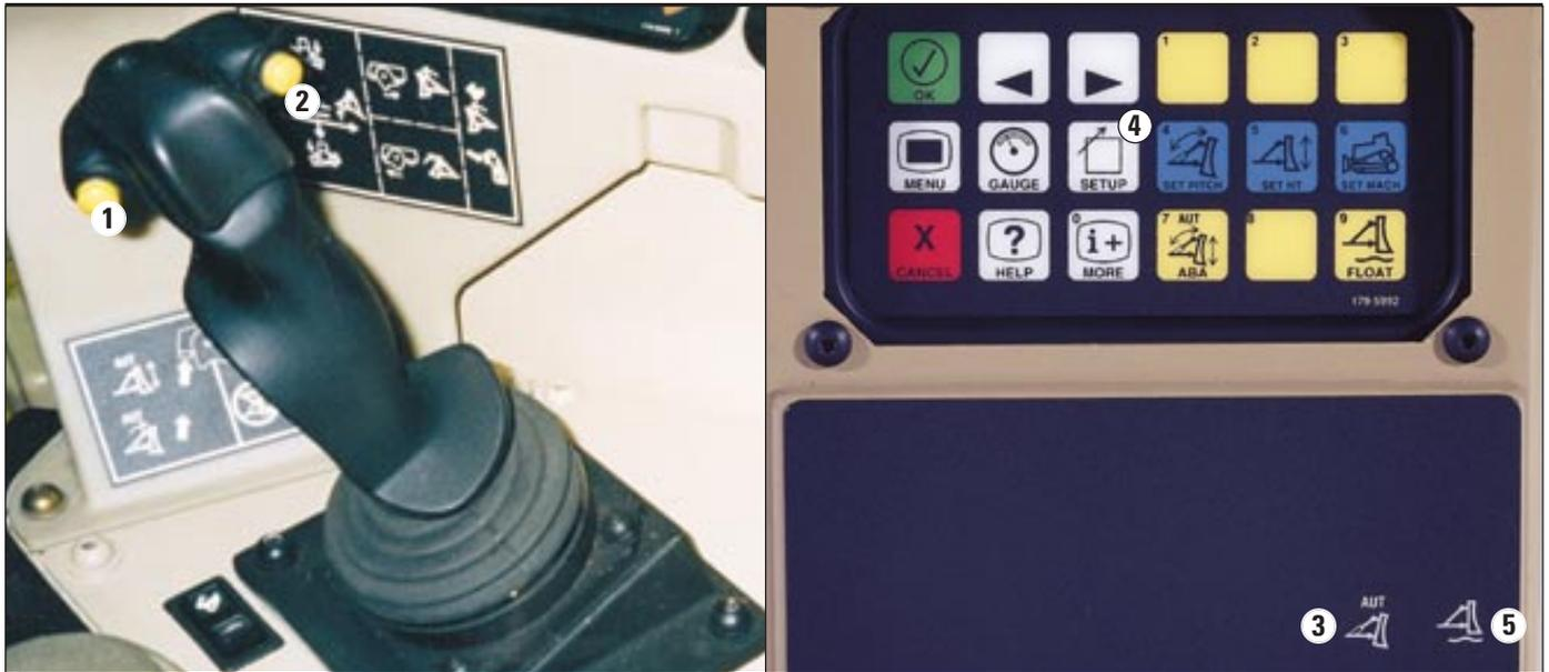
**Automated Blade Assist (ABA)** is a semi-automatic dozer control function that increases efficiency and reduces operator workload by automating some of the more common blade functions. The ABA system for Carrydozer tractors consists of AutoPitch, AutoSpread, and Auto Return.
