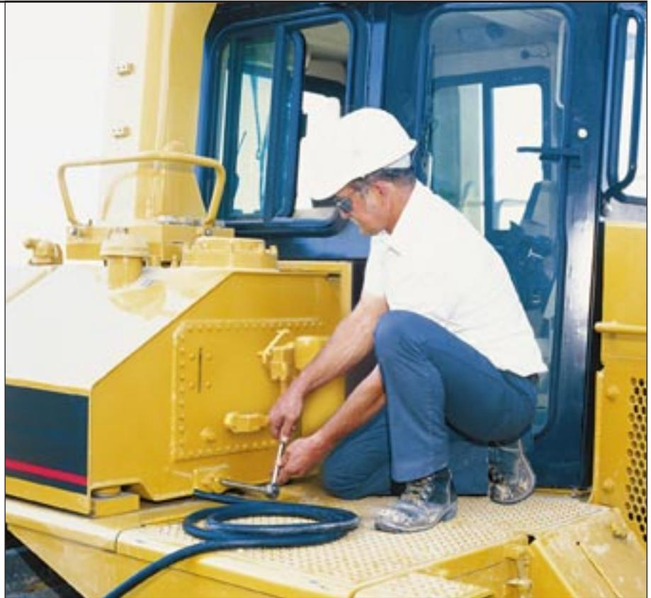
**Ecology drains** provide an environmentally safer method to drain fluids. They are included on the radiator, hydraulic tank and major power train components.
