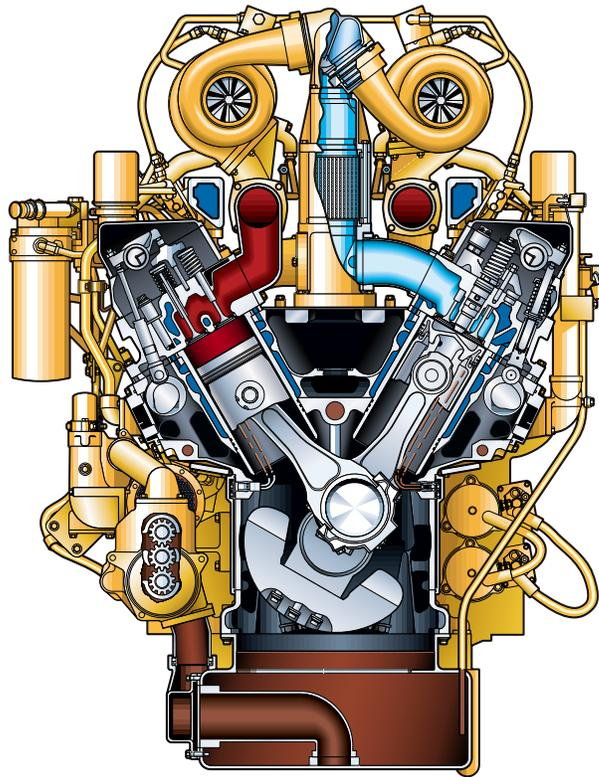
**Caterpillar 3508B Diesel Engine with Electronic Unit Injection (EUI)** performs at rated net power of 634 kW (850 hp) at 1,800 rpm with a torque rise of 25 percent and meets EPA and CARB emissions requirements for 2000.
