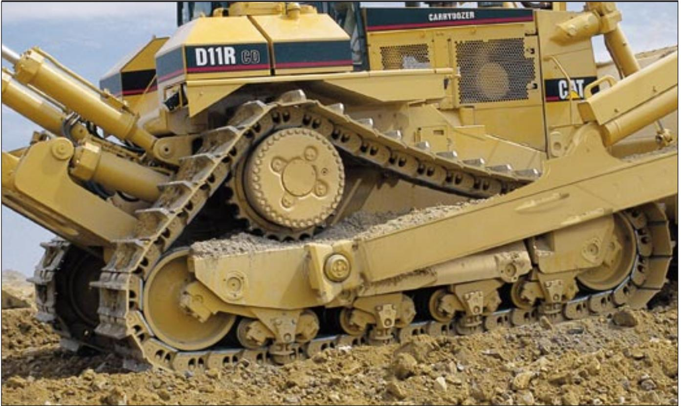
**Suspended undercarriage design** absorbs impact loads to reduce the shock loads transferred to undercarriage by up to 50 percent.
