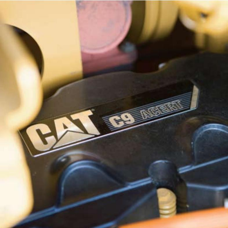
The D7E electric drive train is powered by a 235 hp Cat C9.3 engine with ACERT™ Technology. The engine utilizes a proven common rail fuel system for improved efficiency and fuel economy. Featuring the latest in Cat emissions reduction technologies, this engine meets U.S. EPA Tier III, EU Stage IIIa and Japan MLIT Step 3 emissions regulations.
