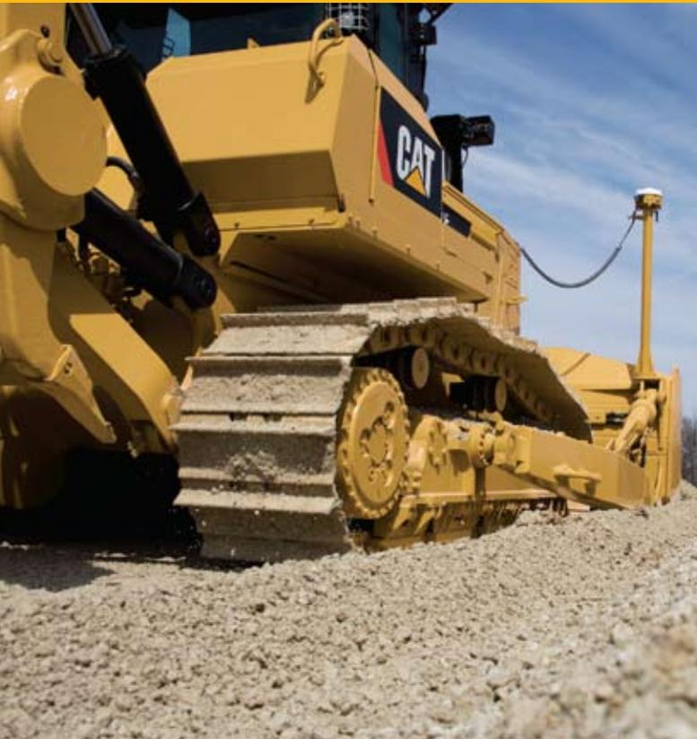
The D7E features an advanced low drive undercarriage design for greater machine versatility in a wider range of applications. Improved visibility, especially to the sides, is only one of the several benefits of this highly efficient undercarriage system.
