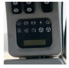
Caterpillar Monitoring System. The 950H is equipped with the Cat Monitoring System (CMS) that keeps watch over the health of your loader. CMS monitors critical engine system functions and will derate the engine to protect itself from damage if needed. Depending on which of the following six critical conditions arise, the CMS monitor or front panel will display warning lights and sound audible alarms.
