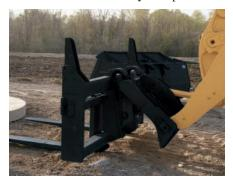
**Quick Couplers.** Quick couplers provide unmatched versatility. The hydraulic model allows an operator to change attachments in seconds without leaving the cab. On the manual model, the operator must lock the pins.
