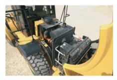
**ENGINE COMPARTMENT ACCESS.** The non-metallic hood on the 950H has been redesigned and restyled from previous models. Side and top panels are stronger due to more robust reinforcement ribs - the change in contour also adds to rigidity of the hood.
