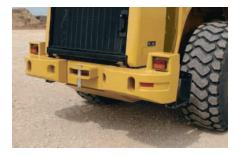
**Counterweight.** The two-piece counterweight is integrated into the 950H design and styling. This 1853 lb (840 kg) counterweight incorporates the rear lights into the top of the structure.
