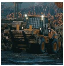
Forestry Applications. The Forest Machine Arrangement provides Ride Control, a heavy-duty tilt cylinder and an additional counterweight for use in forestry and logging applications. Specially-designed work tools for forestry applications can be factory-installed.
