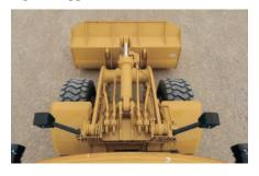
**Linkage.** The 950H linkage is a singletilt Z-bar design. Z-bar linkage generates excellent breakout force and good rack back angle for better bucket loading and load retention.
