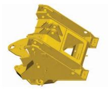
Non-Engine End Frame (NEEF). The non-engine end frame provides a solid mounting base for the front axle, lift arms, lift cylinders and tilt cylinders. The fabricated, four-plate loader tower absorbs the forces associated with loading, twisting and penetration.
