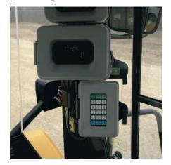
**PAYLOAD CONTROL SYSTEM.** Scales, designed specifically for Cat machines allow on-the-go weighing of material in the bucket. Operators load trucks more accurately and efficiently. Loading trucks right the first time equates to quicker cycles for the operator and more productivity and controllability for your operation.
