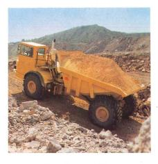
Outstanding Gradeability is provided by the Caterpillar drive train. The D44 can negotiate a total resistance of 40% at a speed of 1.5 mph (2.4 km/h) enabling it to handle the steepest grades and worst site conditions. Users now have more versatility in planning site layout — particularly in mines and quarries. Haul roads can be steeper (and so shorter) giving access to previously uneconomic areas of the job.
