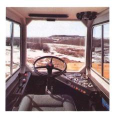
The ROPS/FOPS cab mounted on 'Metalistik' bushes to reduce vibration, provides an ergonomically designed environment for operator efficiency and safety throughout the shift. A full range of easy-to-monitor gauges and warning lights/horn are standard. Visibility is improved by the forward-mounted cab and large window area. Tinted laminated front screen and toughened side screens add to safety.
