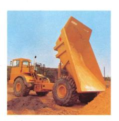
Wide-wedge shaped body design with wrap-around ribs, cushions and reinforces the body against loading shocks. Strength and durability is assured by 145,000 psi (1000 MPa) high-yield, abrasion resistant, heat-treated steel. A 20° ducktail helps retain the load on steep grades. Positioned within the body profile for maximum protection, two double-acting single-stage flex-free hoist cylinders provide fast dump times. A 65° dump angle ensures clean load ejection.
