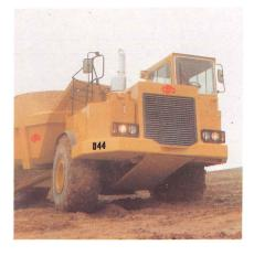
Traction and flotation is outstanding due to large-diameter, wide-base, low pressure radial tires and all-wheel drive. A large foot-print area and equal axle loading keeps the D44 hauling in unbelievable conditions. Tires deflect around obstacles which would penetrate normal high pressure tires. Tire life is extended and haul road maintenance reduced.
