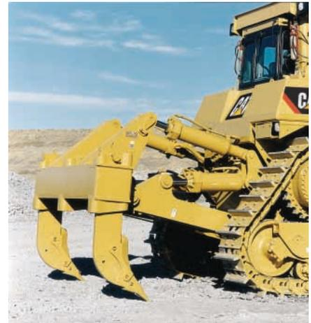
**Multi-Shank Ripper.** Tailors the tractor to the material by using one, two or three shanks.
