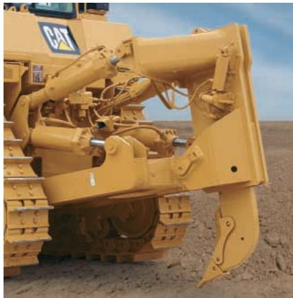
**Single-Shank Ripper.** Operator can adjust the shank depth from the seat using an optional single-shank pin puller. Large upper frame view hole improves ripper tip visibility. Heat treated spacer bars in ripper carriage extend pocket life and reduce shank notching. Large one-piece shank is available in deep ripping configuration.
