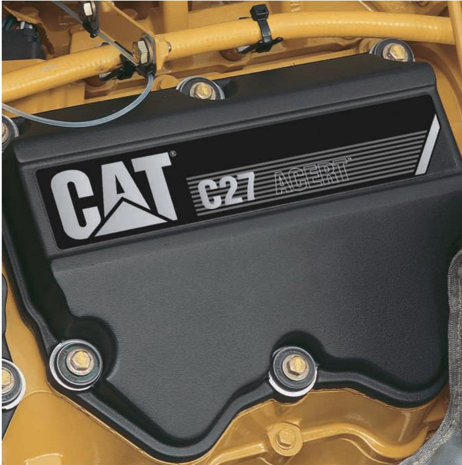
**C27 Engine.** Performing at full-rated net power of 433 kW (580 hp) at 1800 rpm with a high torque rise of 21 percent, the large displacement and high torque rise allow the D10T to doze through tough material. Matched to the high efficiency torque divider and electronically controlled power shift transmission, it will provide years of dependable service.
