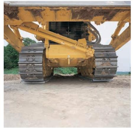
**Tag-Link.** The Tag-Link brings the blade closer to the machine for more precise dozing and load control.
