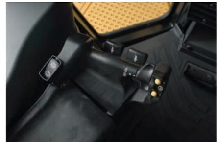
**Finger Tip Controls (FTC).** Clustered for easy, one-hand operation to the operator's left. They control steering, machine direction and gear selection.
