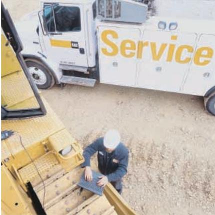
**Serviceability.** Minimizes maintenance and repair downtime. New sight gauges, filter locations, improved access to oil and coolant sampling ports, and an engine compartment mounted work lamp, make daily and periodic service faster and easier. Equipped with a dozer and ripper, there are only 18 lube points.
