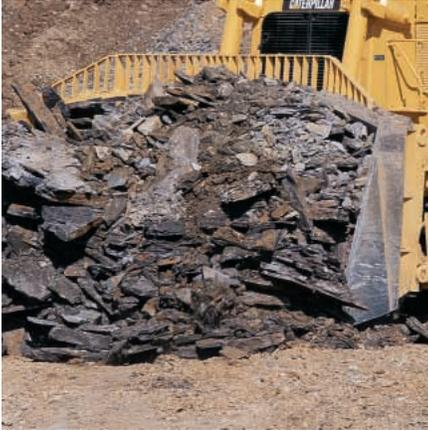
**Bulldozers.** All blades feature a strong box-section design that resists twisting and cracking. Blades are made of Cat DH-2™ steel that has high tensile strength and stands up to the most severe applications. Heavy moldboard construction and hardened bolt-on cutting edges and end bits add strength and durability.
