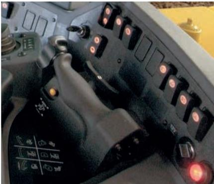
**4) Electronic Ripper Control.** A rigidly mounted handgrip, with low effort thumb and finger controls, provides firm support and positive control of the ripper when operating in tough conditions. Programmable features, such as Auto Lift, Shank-Out and Auto Stow, increase efficiency for the operator.
