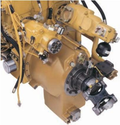
**Torque Divider.** A single-stage torque converter with output torque divider sends 75 percent of engine torque through the converter and 25 percent through a direct drive shaft for greater driveline efficiency and higher torque multiplication. The torque converter shields the driveline from sudden torque shocks and vibration.
