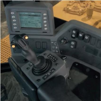
**Dozer Control Lever.** A low-effort electronic dozer control handle gives the operator control of all dozer functions with one hand. Fore/aft movement of the lever lowers and raises the blade. Left/right movement directionally tilts the blade.
