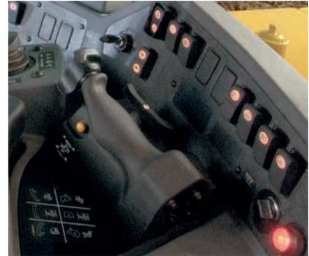
**Ripper Control Lever.** A rigidly mounted handgrip provides firm support for the operator even when ripping in the roughest terrain. The low effort thumb lever controls raising and lowering. The finger lever controls shank-in and shank-out positioning. The thumb button automatically raises the ripper.
