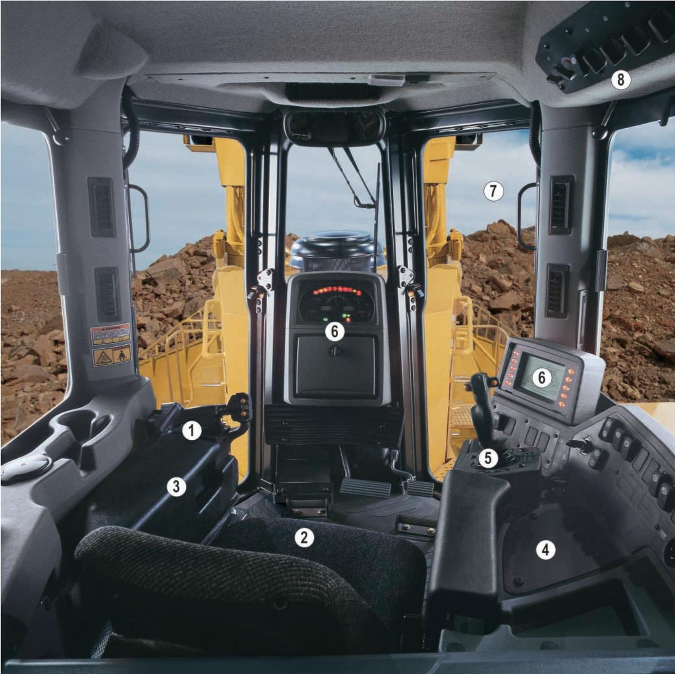
**1) Steering Control.** Finger Tip Control (FTC) combines steering, machine direction and gear selection into a single control system, which can be operated with one hand for enhanced operator comfort.
